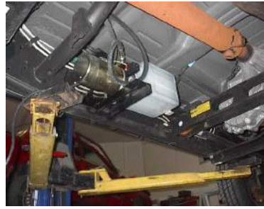
Pump Mounted on Frame
